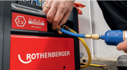
Refrigerant filter for safe recovery included in the scope of delivery
