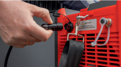
Securely attached power cable
